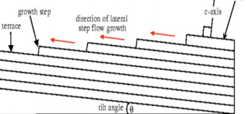
Steps width increases with lowering the temperature ramp
