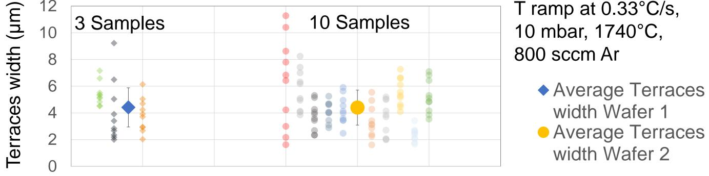
Both wafers are 4H-SiC(0001) on axis, no clear wafer effect
