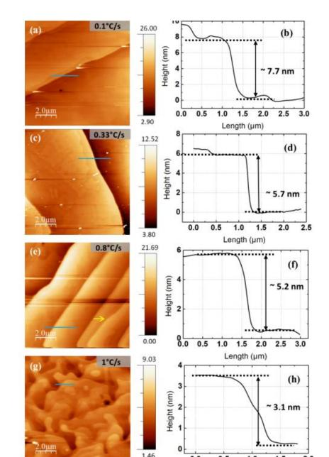
Large terraces up to 20  $\mu$ m with H<sub>2</sub> covered with buffer layer Graphene formation delayed
