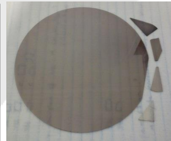
4" LiNbO3 wafer after RTA
